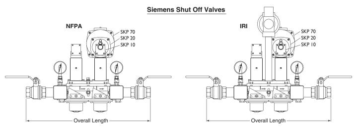
When using the Siemens SKP20 and SKP70 actuators for pressure regulating and ratio regulating functions, the sensing piping is not included. For proper operation, the sensing pipe should be at least 1/4" I.D. and connected a minimum of 5 pipe diameters downstream in a non-turbulent area. WARNING: For proper and safe operation, the installer must read and thoroughly understand the Siemens Technical Instructions 155-514P25 for the SKP20 and 155-516P25 for the SKP70.
